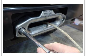
5. Assemble hawse onto M10x1.5x40 mounting bolts and fasten with M10x1.5 flange nuts.
