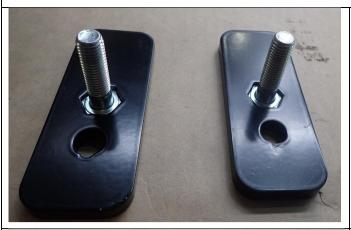
1. Press hex heads of M10x1.5x40 mounting bolts into 8mm thick plates as shown.
