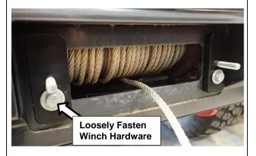
3. Loosely fasten plate & bolt assemblies to lower mounting positions of winch using hardware supplied with winch.
