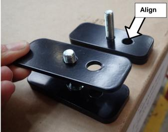
2. Place 4mm thick plates over M10 bolts and align lower 12mm holes.
